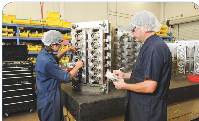
*CSI learned the value of systematic documentation of mold-maintenance procedures and performance issues. Mold data are entered into the MoldTrax5 database for quick generation of custom reports. (Photo: ToolingDocs)*
