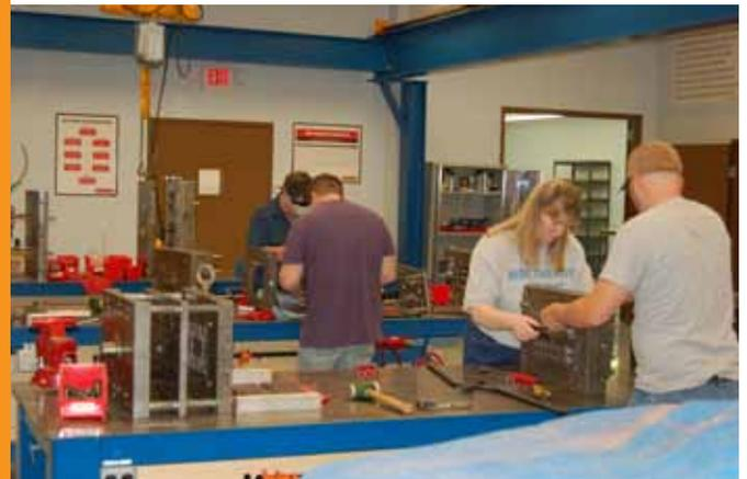
*The design, cleanliness, organization level and general working atmosphere of the shop where mold maintenance work will be done must be taken into consideration. It will help eliminate unnecessary steps and the frustration of hunting for the right tools to do the job.*
